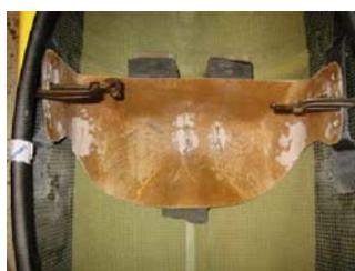
Ensure that the seat is as close to the bottom as possible – a high seat is more unstable than a low seat.
