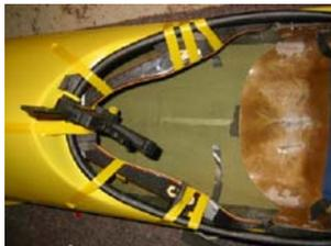
Sit in the boat and fit the thigh braces around you, packing them into position with tape and foam. To ensure good contact cut the bars to fit the contours of the hull. Mark the position for fixing onto the
